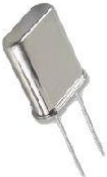
Figure 7.19: Image of a Crystal Oscillator
